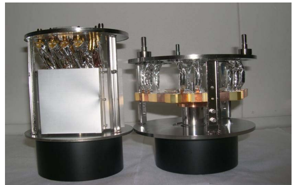
Figure 3: Inside views of the cryogenic rf housings (microenclosures) inside 2004 dewar (left) and 2008 dewar (right). The 2008 dewar has been optimized to eliminate parts as compared to the 2004 design.
